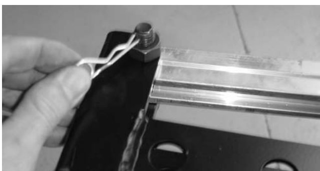
(11) ARCOUPL secured using a locking nut and bolt assembly with cotter pin safety
