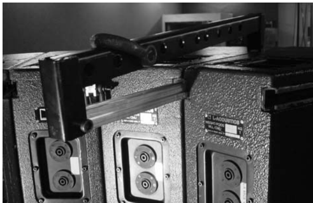
(7) BUMP3 slides into position from the rear
