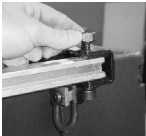
(10) ARCOUPL attached to the main body of the LIFTBAR at the rear
