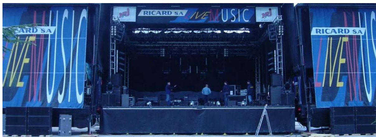
Figure 29: Configuration Stereo in-fill et side fill
