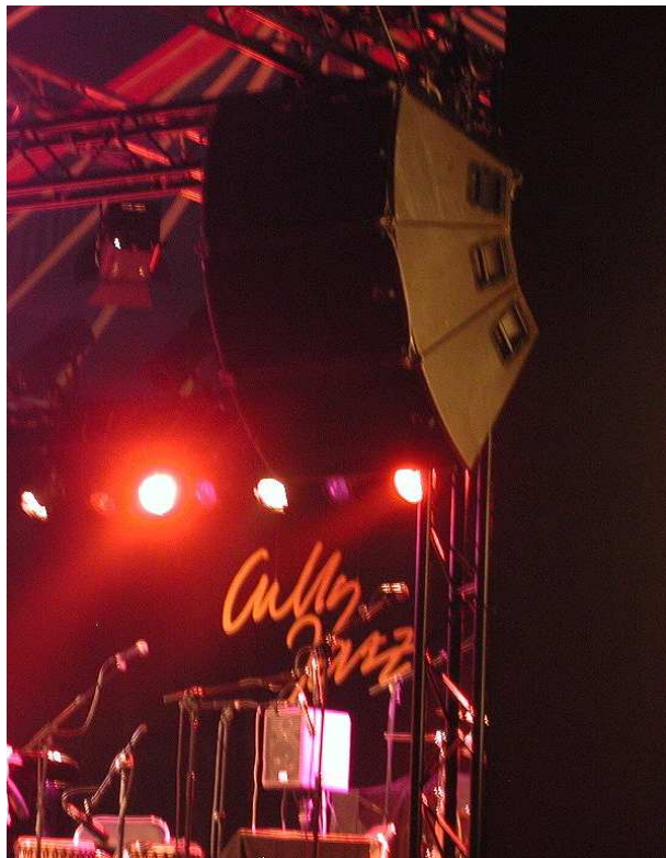
Figure 26: Cluster d'ARCS, orientation horizontale
