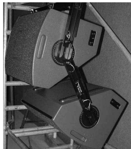
(10) The final installed system. Side flytrack sections and PION2 accessories can be used for installation of safety security steels
