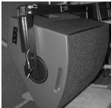
(9) Rotate the pivoting arm into position – the locking pin automatically secures the U-bracket
