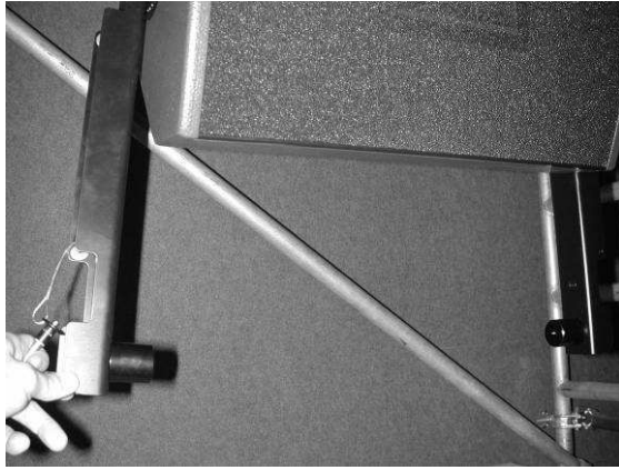
(5) With middle locking pins unattached, the CPL I 12XT is free to rotate, facilitating installation of the lower I 12XT
