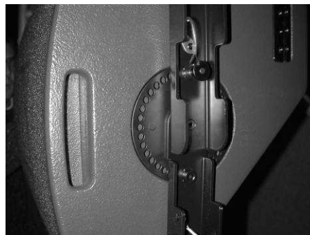
(4) Select angle and secure top locking pins on both sides for the upper I12XT (do not attach middle locking pins for the CPL I12XT)
