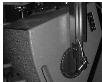
(8) Mount the I12XT in the fixed arm side first
