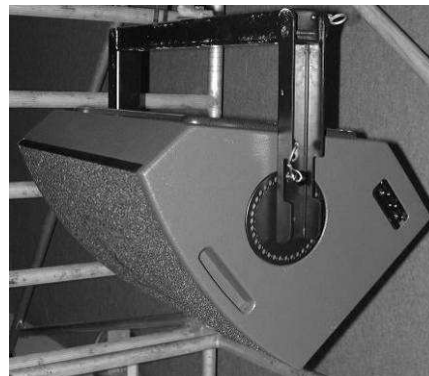
(10) Rotate the loudspeaker into position to select the desired angle. Secure using the locking pins on both fixed and pivoting arms
