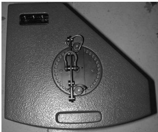
(3) When installing XTLIFTBAR, ensure that the main section is aligned with the center of the enclosure in order to properly balance the center of gravity. The flytrack section and PION2 (optional accessory) can be used to install a safety steel.
