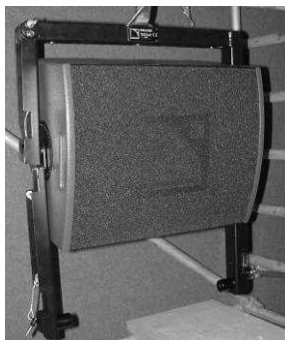
(3) Install the top I12XT. Ensure that the ETRI I2XT rotating arm is properly secured by verifying that the spring-loaded locking pin at the pivot point is correctly seated.
