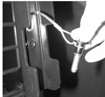
(4) Remove locking pins on both U-bracket arms
