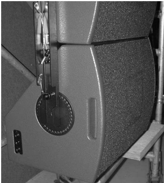
(7) Attach lower locking pins on both sides of the lower I 12XT to facilitate angling of the CPL I 12XT
